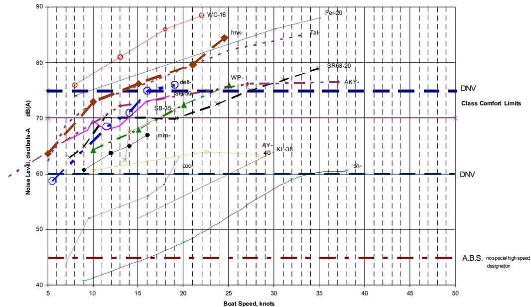
**Fig. 6 Noise Levels in Aft Deck (open) Semi-Displacement & Fast Yachts**
