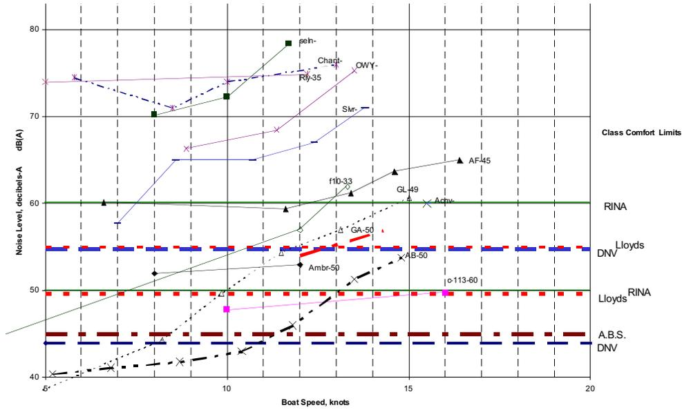
**Fig. 3 Noise Levels in Aft Main Deck & Cockpits (open) Displacement Yachts**
